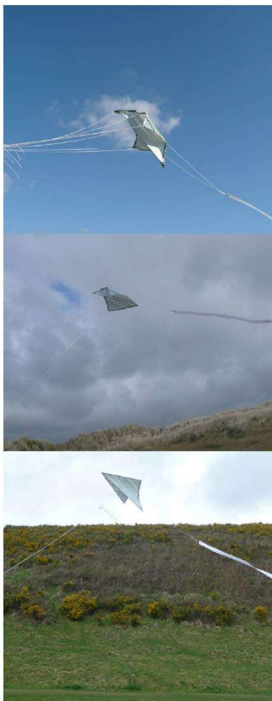
Ref 7. Top: Rogallo replica kite without any stiffening. Middle: Exactly the same kite but with keel stiffening only. Bottom: The same kite but with leading edge and keel stiffening and rigged as a bi-conical wing.
