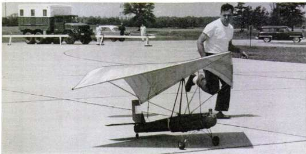
RADIO-CONTROLLED MODEL goes through taxi tests at Langley Research Center of National Aeronautic and Space Administration. The principle of the flexible wing originated with Francis M. Rogallo of the NASA
