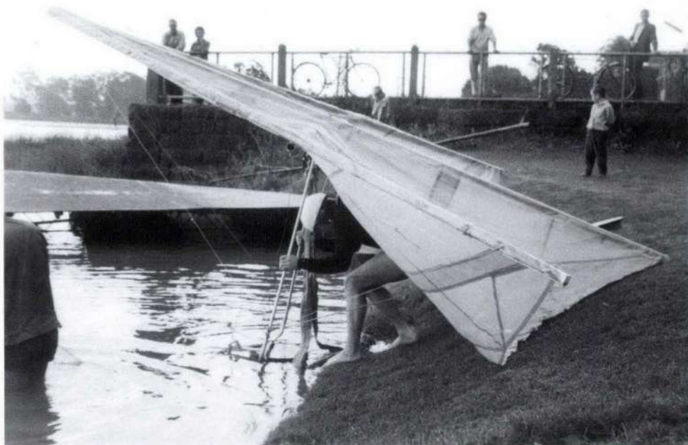
The first of the Mark III gliders. This photo from Grafton shows it in its original configuration. The second set of side wires are visible. The sail is banana bag plastic and insulation tape. John Dickenson is preparing to launch
