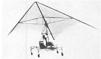
The first prototype of a Ryan Flex-Wing, equipped with 100 HP motor.
