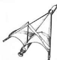
Rogallo wings on rocket. The wings are designed into the rocket assembly. The vanes on the top are for steering.
