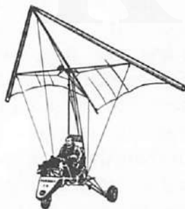
Manned paraglider. This version of the Rogallo has been flown numerous times by several pilots. All flights successful.
