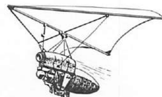
Emergency wings—a parachute substitute. An ejection seat with a jet engine attached enables the pilot to fly with a second set of wings.
