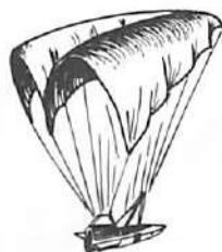
Gliding parachute here being used for towing or drop-launching cargo. Precise landings are controlled by radio signals.
