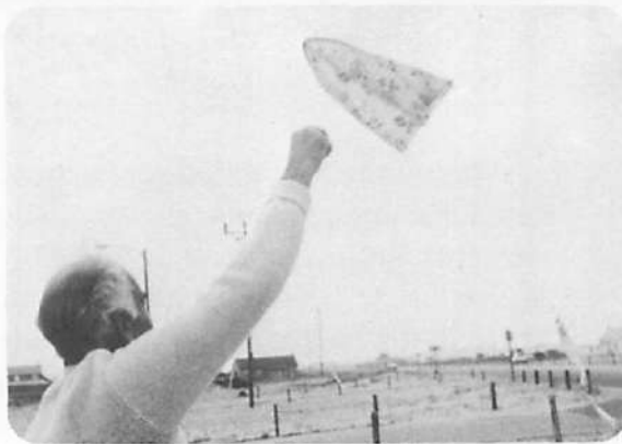
Francis M. Rogallo flies the original 1948 model of the flexible wing. From this flying model the first patents were granted.
