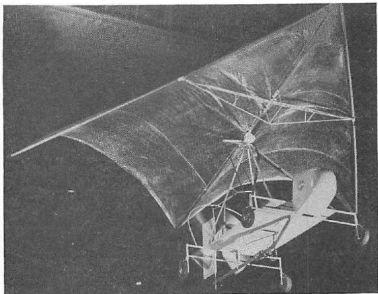
Fig. 1-40. A powered wind tunnel model of a Rogallo wing utility aircraft.
