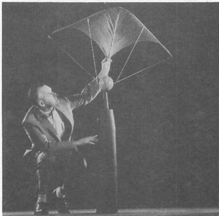
Fig. 1-39. F.M. Rogallo and his flexible wing model with metal keel and leading edges, but no cross bar in the Langley 7 x 10-foot wind tunnel.
