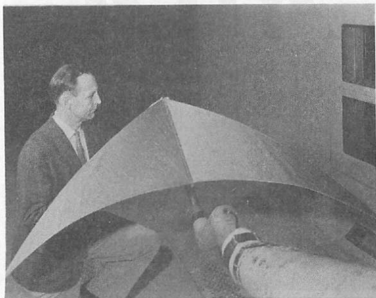
Fig. 1-43. A high aspect ratio cylindrical Rogallo in the Langley 7x10-foot transonic wind tunnel.
